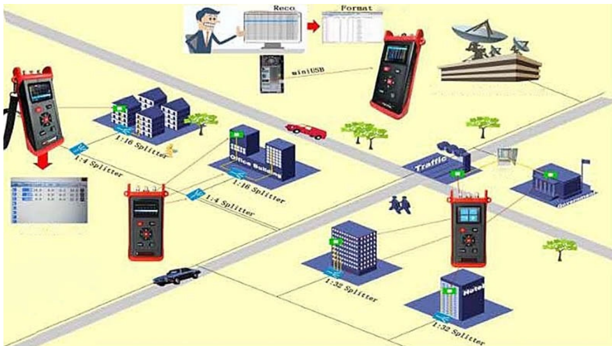
WL-FP01 PON OTDR Application Scenario Diagram
